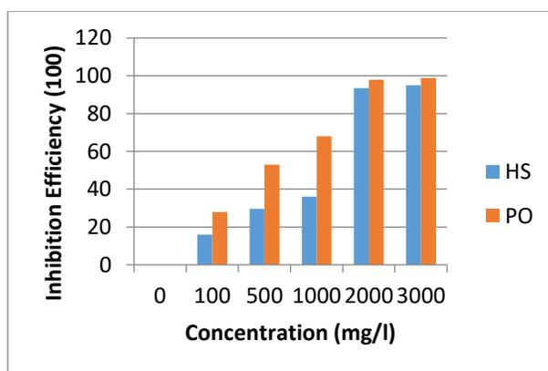
Figure 4: Inhibition Efficiency Rate against concentration of *Pterocarpus osun* and *Hibiscus sabdariffa* for mild steel corrosion in 0.1M HCl at 303K
