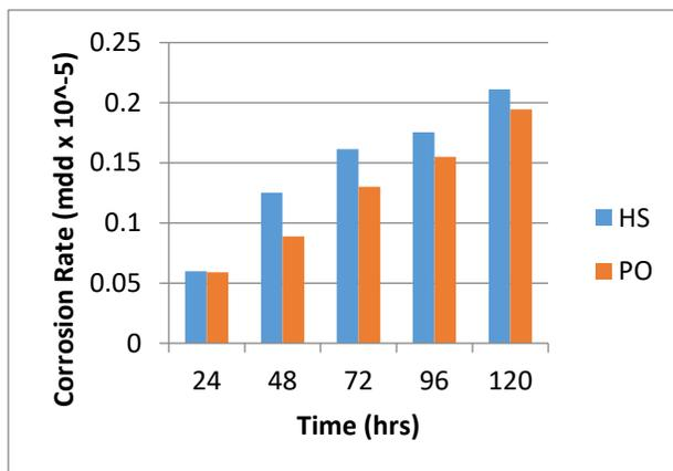
Figure 6: Weight loss against time for mild steel coupons in 1M HCl with or without *Hibiscus sabdariffa* and *Pterocarpus osun* at 303K
