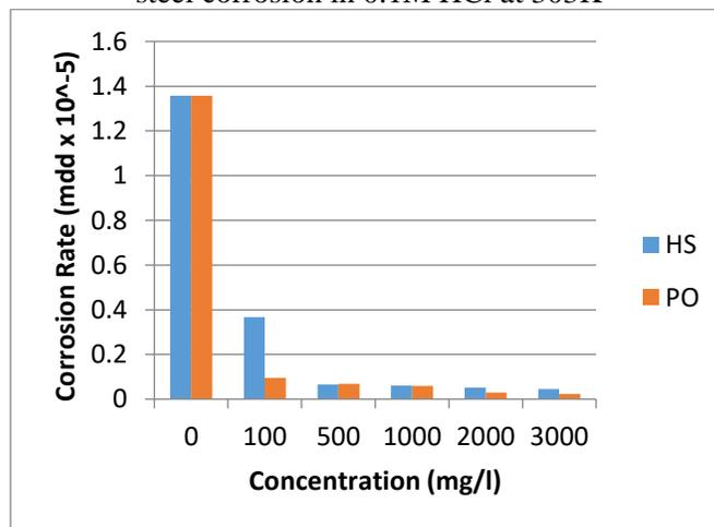
Figure 5: Weight loss against concentration for mild steel coupons in 1M HCl with or without *Hibiscus sabdariffa* and *Pterocarpus osun* at 303K
