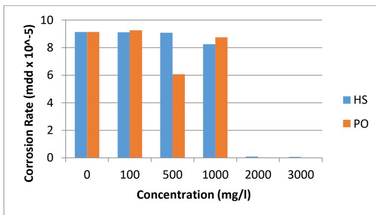
Figure 2: Weight loss against concentration for mild steel coupons in 0.1M HCl with or without *Pterocarpus osun* and *Hibiscus sabdariffa* at 303K
