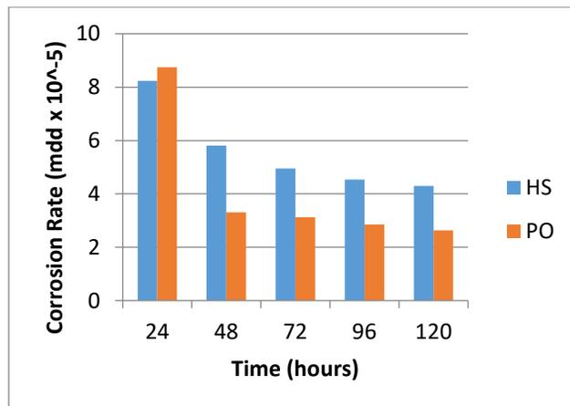
Figure 3: Weight loss against time for mild steel corrosion in 0.1M HCl with or without *Pterocarpus osun* and *Hibiscus sabdariffa* at 303K
