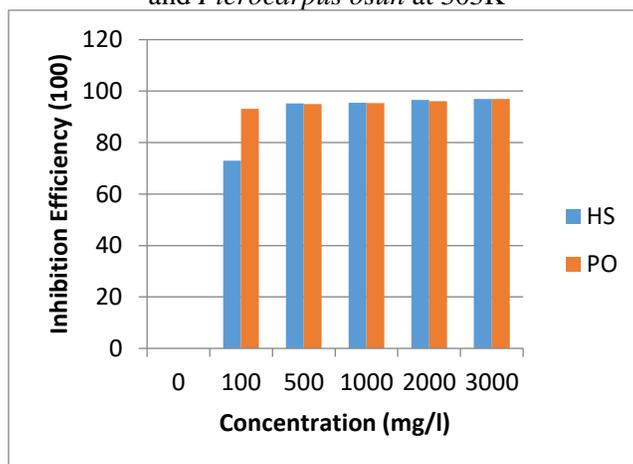
Figure 7: Inhibition Efficiency against concentration of *Pterocarpus osun* and *Hibiscus sabdariffa* for mild steel corrosion in 0.1M HCl at 303K
