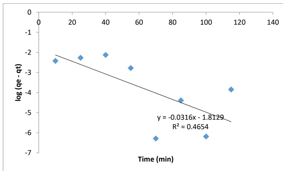
**Figure 8** Pseudo First order kinetics adsorption model of RhB on AMB
