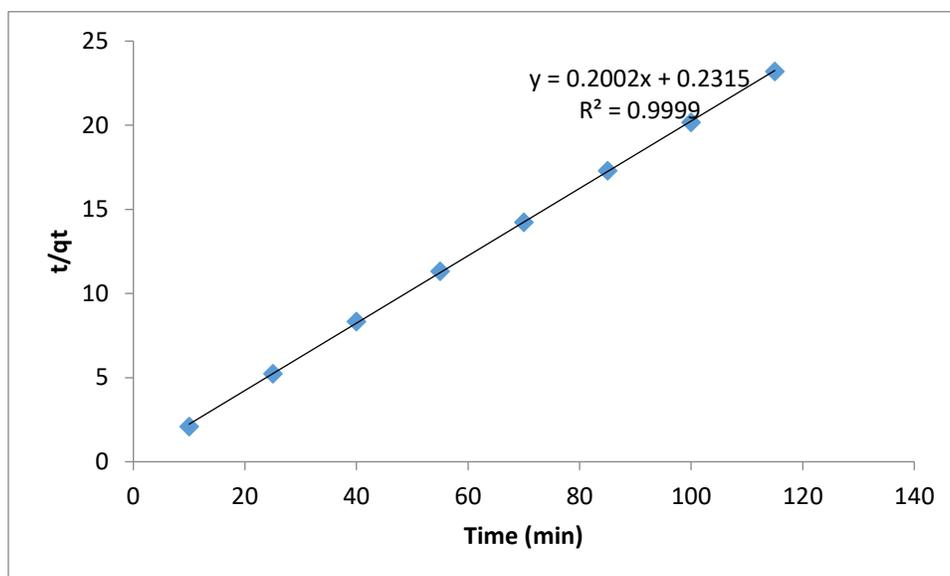
**Figure 9 Pseudo Second order kinetics adsorption model of RhB on AMB**
