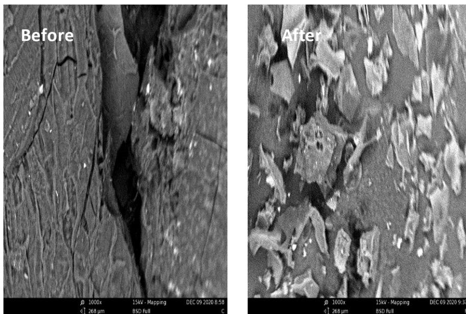
**SEM Images of Modified Biochar Before and After Adsorption (1000× Mag.)**
