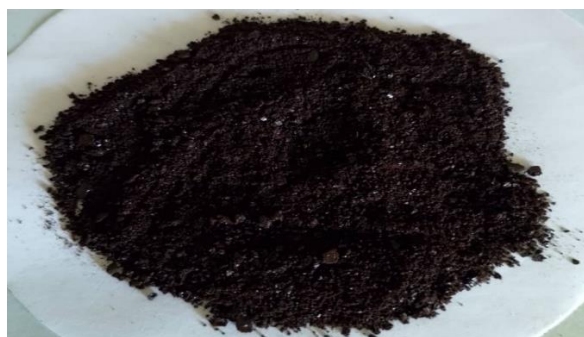
Figure 3. Synthesized \text{Bi}_2\text{O}_3 nanoparticles
